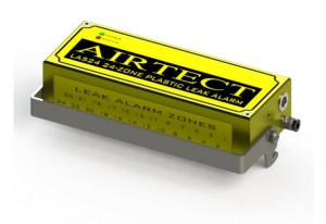
LA524-M-H—N 24-ZONE MODULAR LEAK ALARM MANIFOLD (requires connection to an LA500, LA502 or LM2050 IMM Nozzle Leak Detector Module via a PCC-X Cable. Requires an LA524-B-X base).
